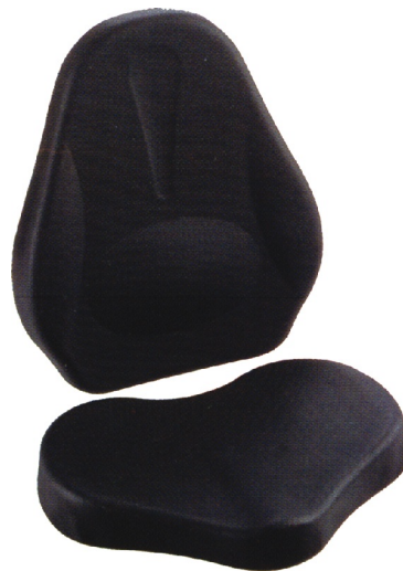
◀ LS-618 Recumbent Seat & Back Seat: 260x420x57mm Back: 327x305x51mm PU self-skinning foam W/ plywood, 8pcs T-nuts Seat: 12PCS/ 3.5CUFT/ 11KGS/ 12KGS Rest: 16PCS/ 3.5CUFT/ 16KGS/ 17KGS
