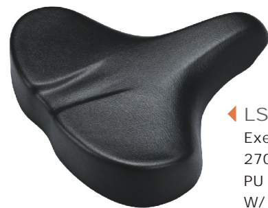
◀ LS-B25 Exercise Saddle 330x324mm PU self-skinning foam, Metal base W/ 3 bolt & nuts or Springs w/steel bracket 20PCS/ 3.84CUFT/ 23.2KGS/ 24.2KGS
