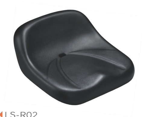
◀ LS-R02 Agriculture seat - Light 400x410x190mm (T=72mm) PU self-skinning foam, Steel frame inner w/ weld nuts 4PCS/ 4.4CUFT/ 13.2KGS/ 14.2KGS
